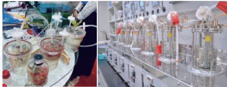
▲ Bio-reactor/ Fermentation air filters
