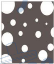
Layer 2 Membrane filter Nylon, PVDF, PTFE, etc. Filters down to 0.45\ \mu\text{m} or 0.2\ \mu\text{m}
